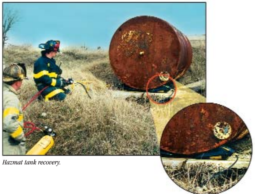
Lift and level pipelines not accessible to heavy equipment.
