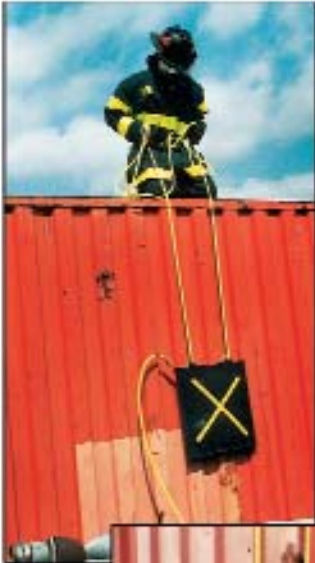
Vertical placement using positioning eyelets.
